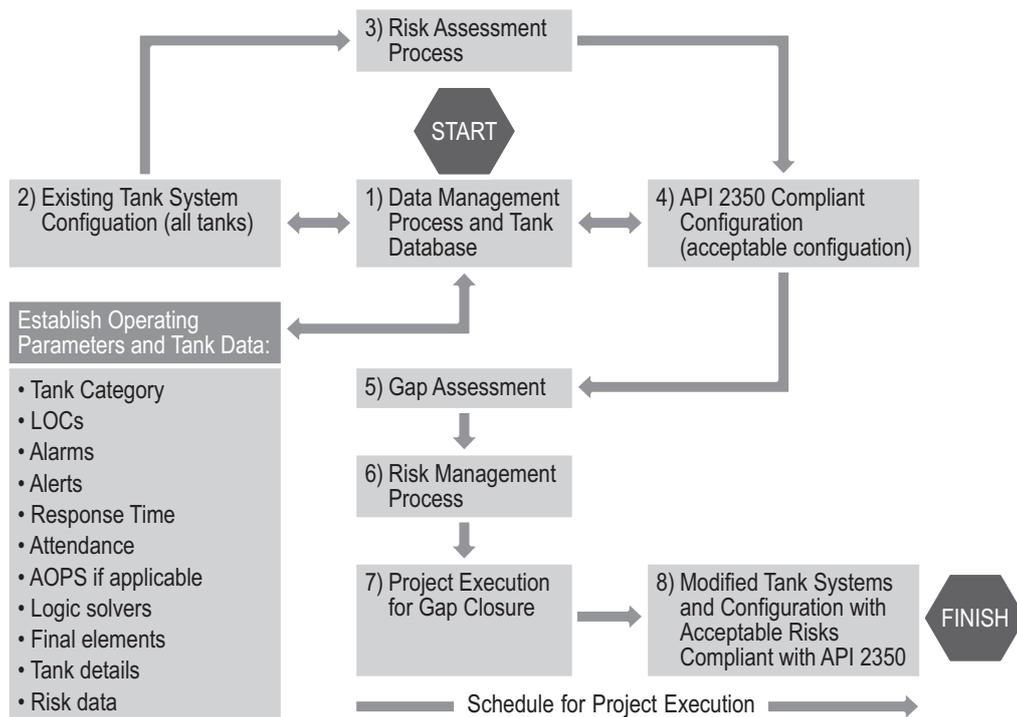
**Figure 1: Conceptual Management Plan for Implementation of API 2350**
