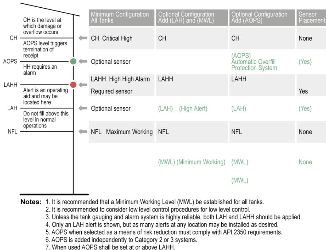
**Figure 3: API 2350 Tank Levels of Concern (LOCs) – Category 2 and 3 Configurations**
